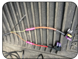
Two Add-A-Fuse Holders Assembled on CYL-V Power and Ignition Wires
