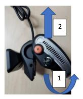
(1) Swing the recorder from the bottom upwards until resistance is felt, (2) then push up
