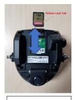
Remove the card by pushing down into the slot. The card will pop up
