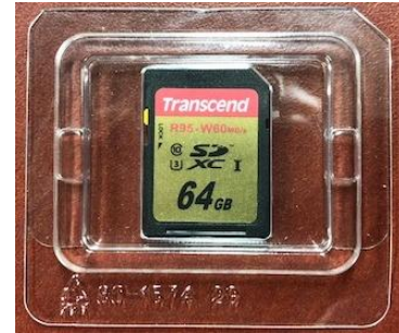
DV453: SD CARD 64GB SD card (DV453) – changed from 32GB to 64GB since mfg. date code 1703
