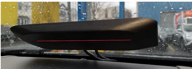
Fig 3. Bottom Side Windshield Mount Antenna (Interior View)
