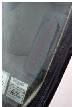
Fig 2. Left Side Windshield Mount Antenna (Outside View)
