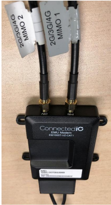
Fig 5. Connect MIMO1 to PRI port & MIMO2 to DIV port in the modem
