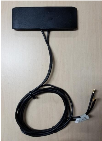
Fig 4. If the antenna wire is too long, bundle it round and use a couple of zip ties to secure the cable
