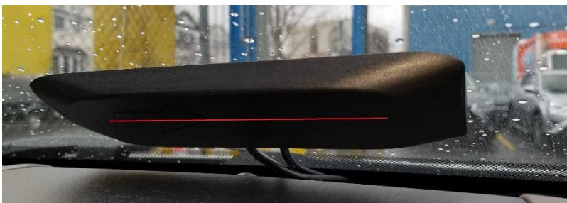
Fig 3. Bottom Side Windshield Mount Antenna (Interior View)
