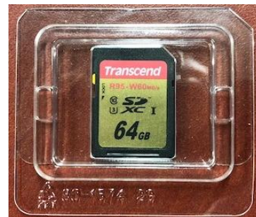
DV453: SD CARD 64GB SD card (DV453) – changed from 32GB to 64GB since mfg. date code 1703
