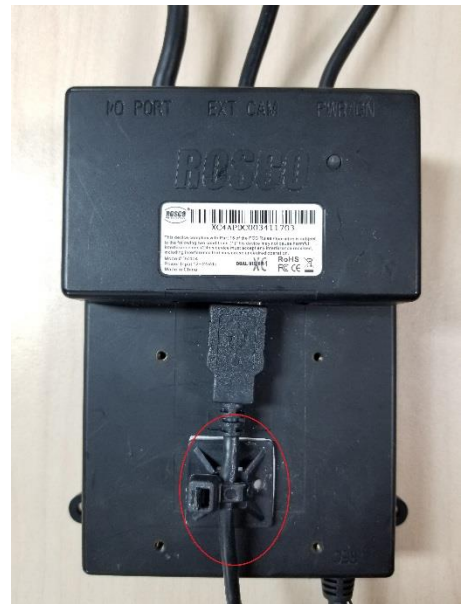
Fig 6. Use a zip tie (TIE1001) and secure the USB cable on PDC
