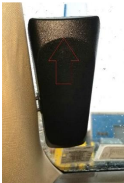
Fig 1. Left Side Windshield Mount Antenna (Interior View)
