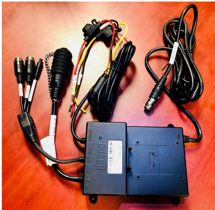
DV403P: PDC MODULE ( Power and Data Control )
