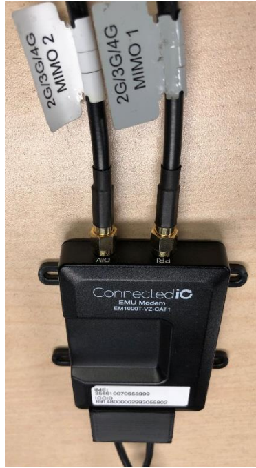
Fig 5. Connect MIMO1 to PRI port & MIMO2 to DIV port on the modem
