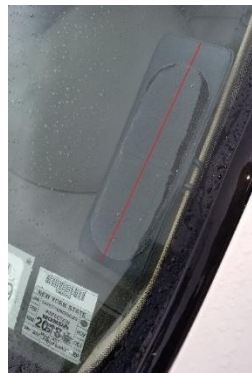
Fig 2. Left Side Windshield Mount Antenna (Outside View)
