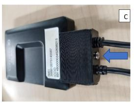
Connect the MIMO 2 antenna wire to the Modems DIV connector
