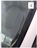
Notice the angled part of the antenna is on the *inside* of the vehicle (Photo A & B). Make sure the FLAT SIDE of the antenna has a CLEAR VIEW OF THE SKY and is facing OUTSIDE (Photo C)
