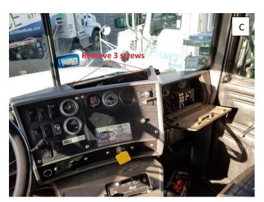
The PDC & Modem are mounted on the top of the dash in the center cavity.
