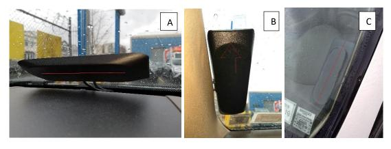
Notice the angled part of the antenna is on the *inside* of the vehicle (Photo A & B). Make sure the FLAT SIDE of the antenna has a CLEAR VIEW OF THE SKY and is facing OUTSIDE (Photo C)
