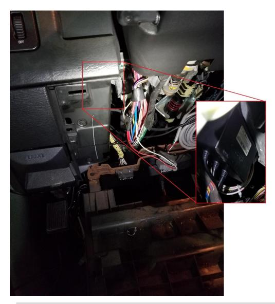
IT'S IMPORTANT TO NEATLY ZIP TIE WIRES TO A FACTORY BRACKET OR HARNESS TO PREVENT FROM FALLING. KEEP AWAY FROM THE STEERING FUNCTIONS AND ANY MOVING PARTS
