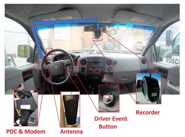
Before starting your installation, please take note of component mounting locations. Follow the blue arrow for recorder cable routing
