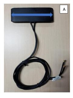
After all connections are made, coil up all the extra antenna cable (Photo A)
