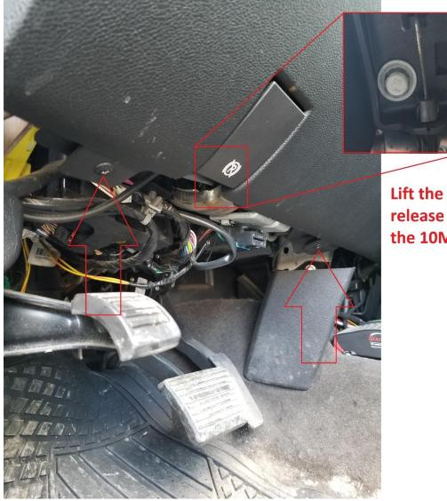
Lift the parking brake release latch to access the 10MM bolt
