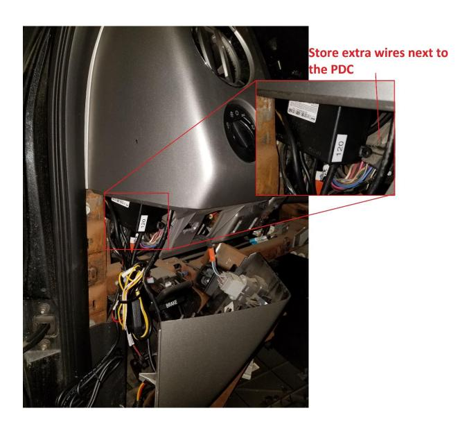
IT'S IMPORTANT TO NEATLY ZIP TIE WIRES TO A FACTORY BRACKET OR HARNESS TO PREVENT FROM FALLING. KEEP AWAY FROM THE STEERING FUNCTIONS AND ANY MOVING PARTS
