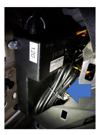
IT'S IMPORTANT TO NEATLY ZIP TIE WIRES TO A FACTORY BRACKET OR HARNESS TO PREVENT FROM FALLING. KEEP AWAY FROM THE STEERING FUNCTIONS AND ANY MOVING PARTS
