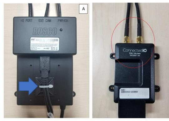
Connect the MIMO 1 antenna wire to the Modems PRI connector
