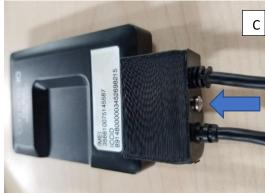
Connect the MIMO 2 antenna wire to the Modems DIV connector
