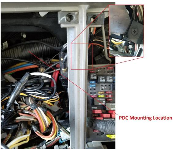
IT'S IMPORTANT TO NEATLY ZIP TIE WIRES TO A FACTORY BRACKET OR HARNESS TO PREVENT FROM FALLING. KEEP AWAY FROM THE STEERING FUNCTIONS AND ANY MOVING PARTS
