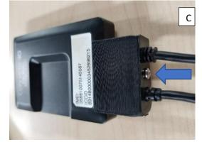
Connect the MIMO 2 antenna wire to the Modems DIV connector
