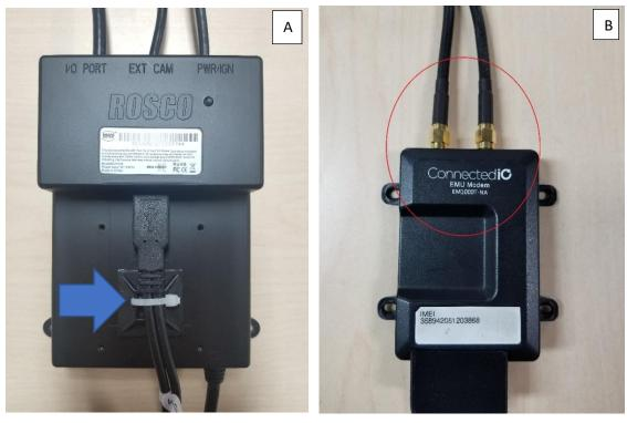
Connect the MIMO 1 antenna wire to the Modems PRI connector
