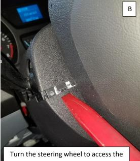
Turn the steering wheel to access the clip on the other side
