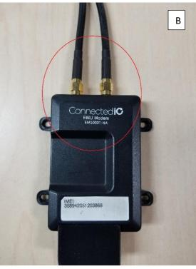
Connect the MIMO 1 antenna wire to the Modems PRI connector
