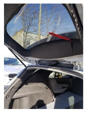
Route the video cable down the passenger side of the vehicle and connect to the C3 of the PDC
