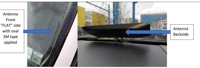
Notice the angled part of the antenna is facing down (Photo A & B). Make sure the FLAT SIDE of the antenna has a CLEAR VIEW OF THE SKY and is facing OUTSIDE (Photo C)
