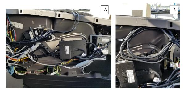
IT'S IMPORTANT TO NEATLY ZIP TIE WIRES TO A FACTORY BRACKET OR HARNESS TO PREVENT FROM FALLING. KEEP AWAY FROM THE STEERING FUNCTIONS AND ANY MOVING PARTS
