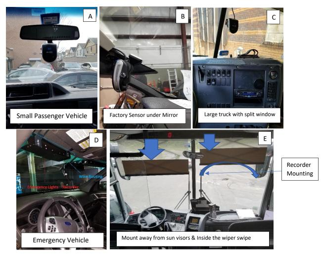
For small passenger vehicles, mount the Recorder under the rear-view mirror (Photo A).
