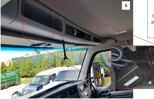
Make sure all extra wire slack is stored away from the CB Radio cavity! Secure all wires with zip ties behind the storage pockets
