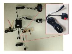
With a driver event button located on the Recorder (Right side of the driver), its best to place the external driver event button on the left side of the driver
