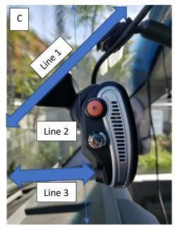
Line 1 represents the angle of the windshield. Line 2 represents the Recorder angle. Line 3 represents the location of the lens. Notice line 2 is slightly angled. This is to capture the front of the vehicle.
