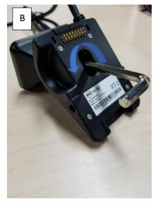
When the Pedestal and cradle hit the tool (Blue Arrows in Photo C), tighten the Alan Key by turning clockwise
