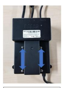
After the WIFI adapter is plugged into the USB port of the PCD, secure the mount cover with the 4 Philips screws
