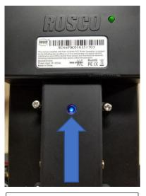
When the PDC is powered up verify the blue LED light is on and flashing. This will confirm the adapter is installed correctly
