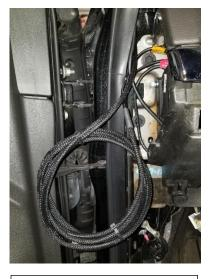
Coil the extra antenna cable and store it in a safe location next to the PDC. NEVER BEND THE EXTRA CABLE
