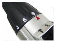
Use a low clutch setting on your drill to prevent overturning
