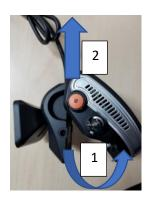
(1) Swing the recorder from the bottom upwards until resistance is felt, (2) then push up
