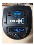
If the SD card is installed incorrectly you will see "nOSd"
