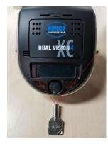
Unlock the 2 locks on both sides of the recorder
