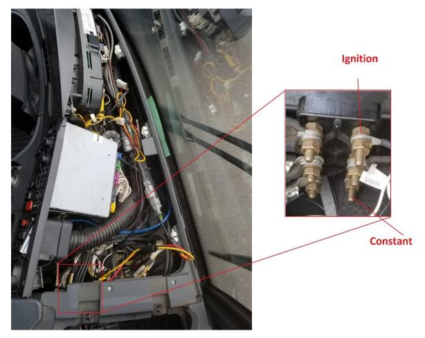
This vehicle has a multiplexer which causes a power delay. When the vehicle is powered down, the recorder will stay powered up for 30 seconds to one minute before switching to parking mode
