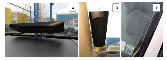
Notice the angled part of the antenna is on the *inside* of the vehicle (Photo A & B). Make sure the FLAT SIDE of the antenna has a CLEAR VIEW OF THE SKY and is facing OUTSIDE (Photo C)
