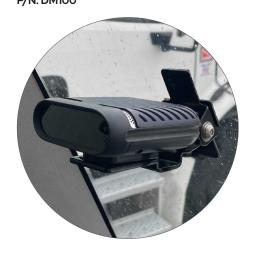
Rosco's new Driver Management System (DMS) uses the latest AI to track driver's eyes and head positions for signs of drowsiness and distraction. Prevent an event before it happens with the most accurate AI in the fleet management market.
